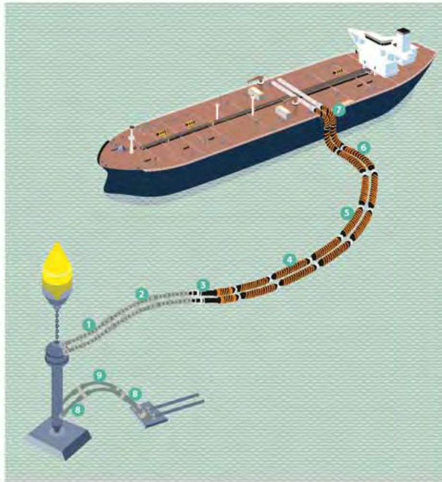
Example of Hoses in a SALM System (Refer to Table 14 overleaf)
